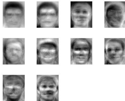
Fig. 3 b). First 10 eigenfaces or eigenvectors corresponding to the first 10 eigenvalues of a sample collection of images
