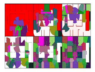
Fig. 10. 25 nodes in a moderately-complex environment. The first three images show the nodes running the Sentinel algorithm. Once the environment has been explored, the nodes switch to a Voronoi-region based static coverage algorithm, shown in the bottom three images. Lines between two nodes show when nodes are able to communicate with each other.
