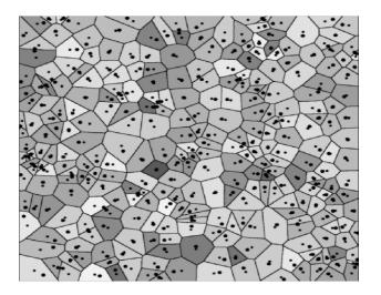
Fig. 1. Voronoi diagram with generators (large dots) and centroids (small dots)[6]
