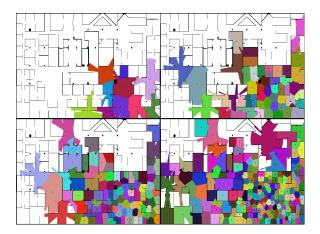
Fig. 7. Placement and coverage of 10, 50, 100, and 200 nodes using a Voronoi-region based static coverage algorithm.
