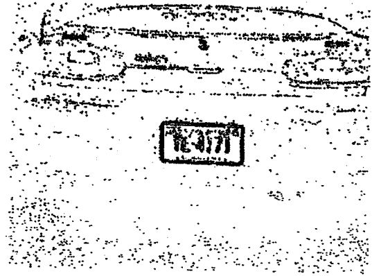
Figure 4. Edge detection of photo #90 using Robert's Cross matrix
