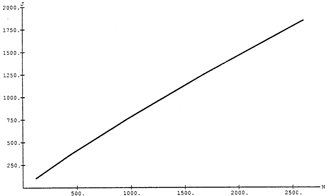
Figure 2: The number of Jacobi iterations for convergence (normalized \ell_2 -norm less than \leq 1.0 \times 10^{-3} ); N is the total number of grid points in the finite element mesh and J is the number of Jacobi iterations required for convergence.
