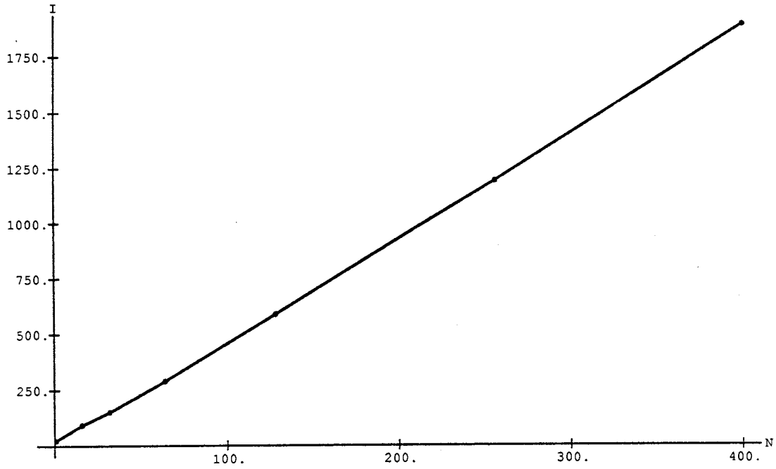
Figure 6: Number of conjugate gradient iterations (I) required for the normalized global residual to reach a value \leq 1.0 for various discretizations (N) in the width dimension.
