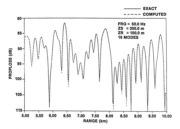
Figure 3: Pade(2,2) test results for 16 propagating modes. Solid line = exact solution, dashed line = computed solution.
