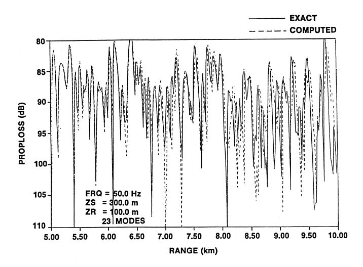
Figure 2: Pade(2,2) test results for 23 propagating modes. Solid line = exact solution, dashed line = computed solution.
