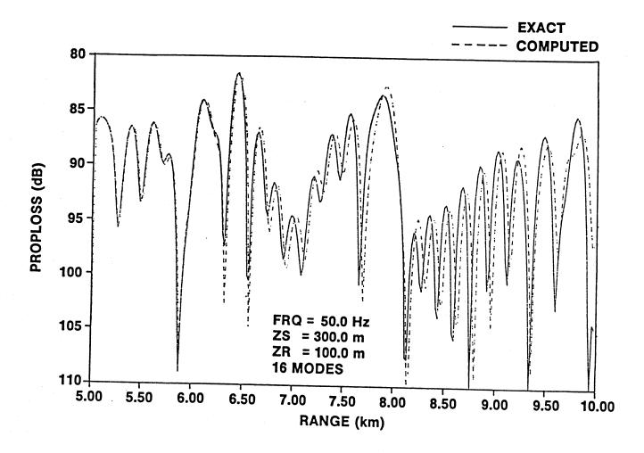
Figure 1: Pade(1,1) test results for 16 propagating modes. Solid line = exact solution, dashed line = computed solution.
