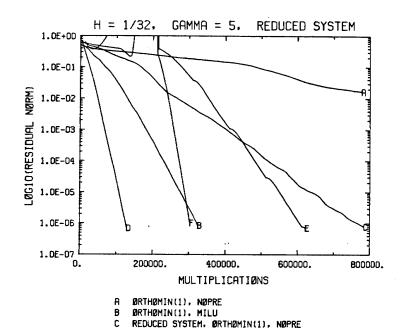
Figure 11-5: Reduced system preconditioning, and reduced system followed by MILU preconditioning, compared with methods applied to the full linear system, for γ=5, h=1/32.
