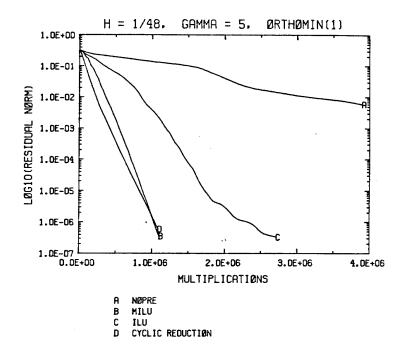
Figure 11-4: Residual norm vs. multiplications for Orthomin(1) with several preconditionings and with no preconditioning, for  $\gamma=5$ , h=1/48.
