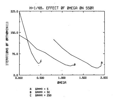
Figure 11-22: The effect of w on SSOR preconditioning, for h=1/48.
