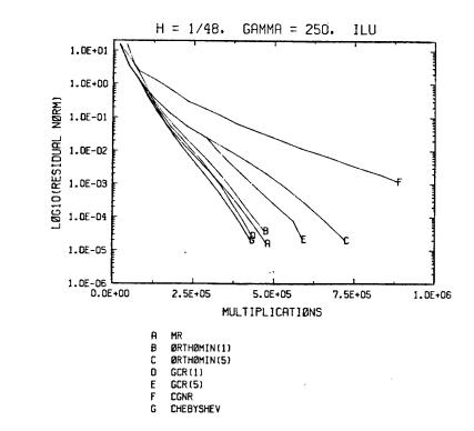
Figure 11-16: Residual norm vs. multiplications for several iterative methods with ILU preconditioning, for  $\gamma$ =250, h=1/48.
