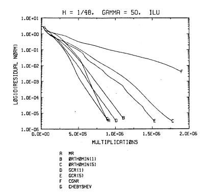
Figure 11-9: Residual norm ws. multiplications for several iterative methods with ILU preconditioning, for  $\gamma=50$ , h=1/48.
