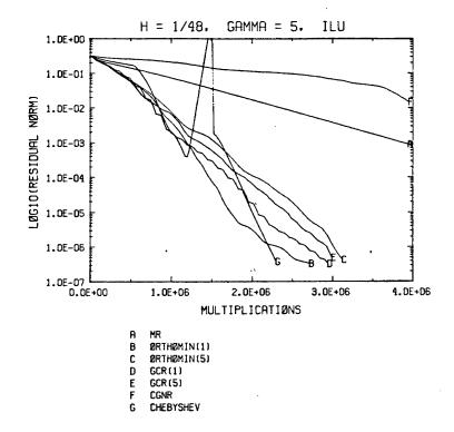
Figure 11-2: Residual norm vs. multiplications for several iterative methods with ILU preconditioning, for  $\gamma=5$ , h=1/48.
