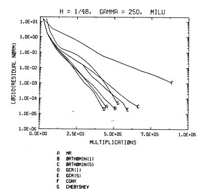
Figure 11-15: Residual norm ws. multiplications for several iterative methods with MILU preconditioning, for  $\gamma$ =250, h=1/48.
