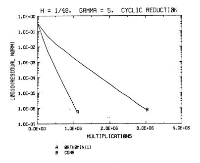
Figure 11-3: Residual norm vs. multiplications for several iterative methods with cyclic reduction preconditioning, for  $\gamma=5$ , h=1/48.
