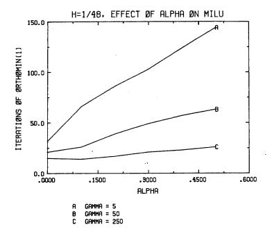
Figure 11-21: The effect of a on MILU preconditioning, for h=1/48.
