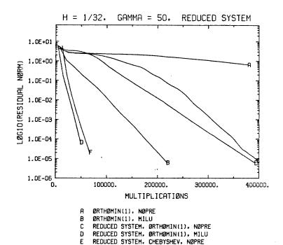
Figure 11-12: Reduced system preconditioning, and reduced system followed by MILU preconditioning, compared with methods applied to the full linear system, for  $\gamma$ =50, h=1/32.
