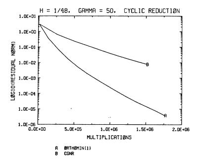
Figure 11-10: Residual norm vs. multiplications for several iterative methods with cyclic reduction preconditioning, for  $\gamma=50$ , h=1/48.
