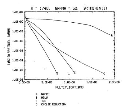
Figure 11-11: Residual norm vs. multiplications for Orthomin(1) with several preconditionings and with no preconditioning, for  $$\gamma = 50$$  , \$h = 1/48\$ .
