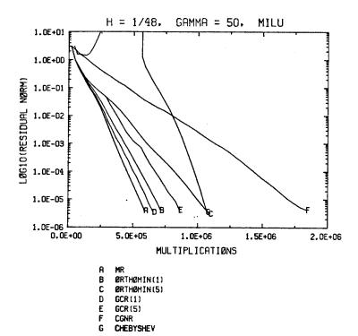
Figure 11-8: Residual norm vs. multiplications for several iterative methods with MILU preconditioning, for  $\gamma$ =50, h=1/48.
