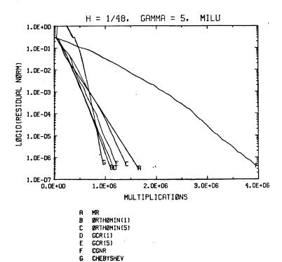
Figure 11-1: Residual norm ws. multiplications for several iterative methods with MILU preconditioning, for  $\gamma=5$ , h=1/48.
