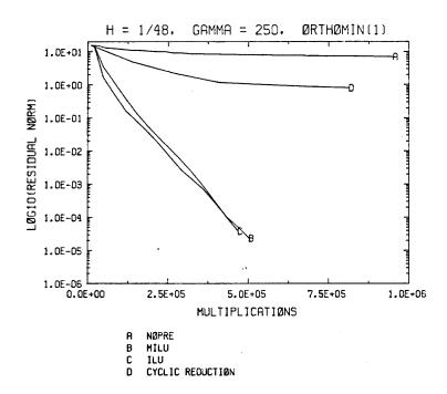
Figure 11-17: Residual norm vs. multiplications for Orthomin(1) with several preconditionings and with no preconditioning, for  $\gamma$ =250, h=1/48.
